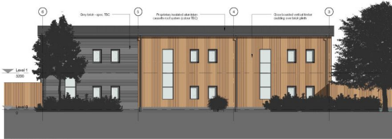
Units 6 - 8 North Elevation 1:100
